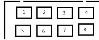
The **Ctrl port** has 8 pins, it is not necessary for the installers to use it in most cases, however it can be used for installer's convenience in case many more extra devices are installed.
